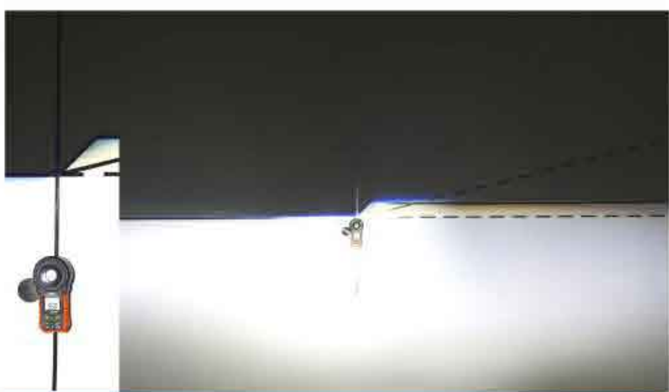
LOW BEAM PROJECTOR/3500LUX
